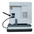
6 Connect the DC In jack of the External Battery Kit with a suitable DC source, e.g. the power supply that is delivered with the 4274 DC Option.
