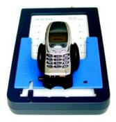
The important feature with the Antenna Coupler is that mobile phones of the same type are always placed in exactly the same position in the clamp.
