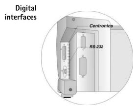
The 4200 includes a D sub-25 socket to connect to a printer (Centronics interface) and a D sub-9 socket to connect to a PC (serial or RS-232 interface). See the user guide for a description of different applications.
