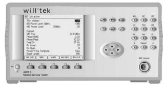
The main elements of the 4200 are the front panel with an LCD screen, keys and the RF connector, the mains connector at the right-hand side and the digital interface connectors at the back.
