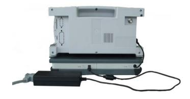
Charging the The 4281 External Battery Kit includes a preinstalled, rechargeable battery lithium-ion (Li-Ion) battery. A fully charged battery is good for two to three hours of continuous use.
