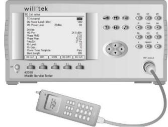
**Points in favor** RF adapter with cable coupling guarantees a set of defined testing conditions. That means that all tests produce results which can be correctly evaluated against specifications.
