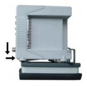
4 Turn the clamps over the 4200 so that the 4200 is safely held on top of the External Battery Kit.
